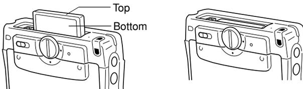
Carefully slide the card into the slot as far as it will go.
