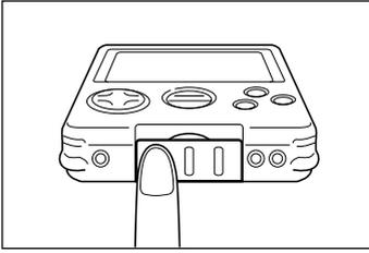
Press one side of the serial connector cover with your finger.
