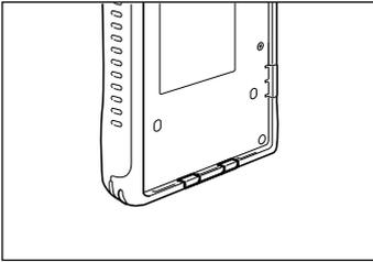
Check again to make sure that the serial connector cover is laying flat without any gaps around its edges.
