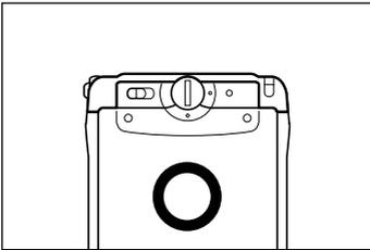
Proper and complete sealing
