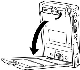
4. Insert the bottom edge of the new battery pack into the groove at the bottom of the battery compartment, and then swing the top of the battery pack into place.
