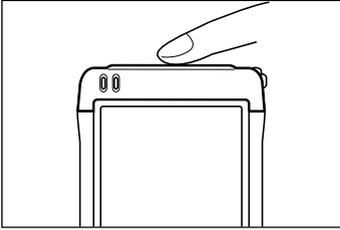
Finally press the center of the cover and check to make sure that it closes completely.
