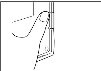
If the raised part of the jack cover is not completely inside of the groove, press it into place by running your fingertip along the cover.
