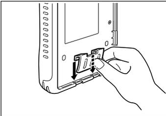
Serial connector cover removed
