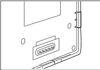
Check to make sure that the entire jack cover is completely and correctly pressed into the case.
