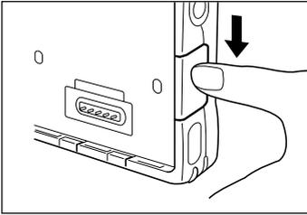
Press down on one side of the jack cover and then slide your finger to the other side so it completely closes.
